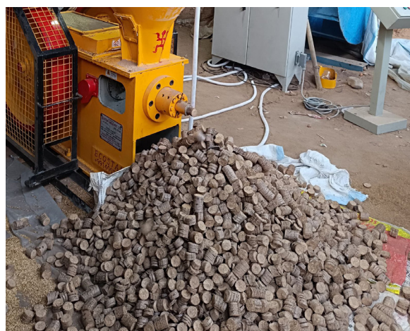
Figure 64: Briquettes manufactured from agricultural waste
